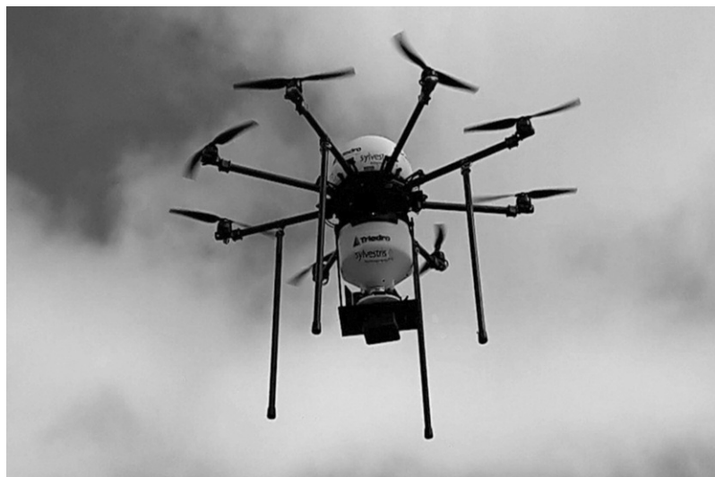
Picture 5: Octocopter seeder developed by TRIEDRO and SYLVESTRIS. © F. Martínez Sanz.
