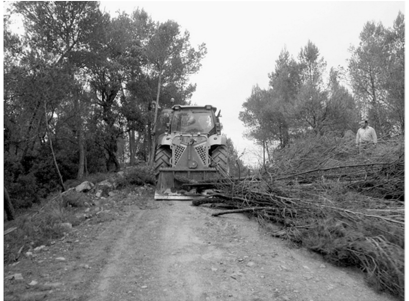
Picture 4: Agricultural tractor with load. On average, each rotation ensured the skidding of 12 trees.
